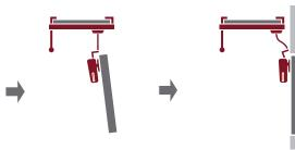
Use console clip to move window towards window opening and trigger the pivot-arm during mounting.
