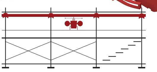
The SnapClamp is open in the bottom allowing the trolley to move through the SnapClamp
